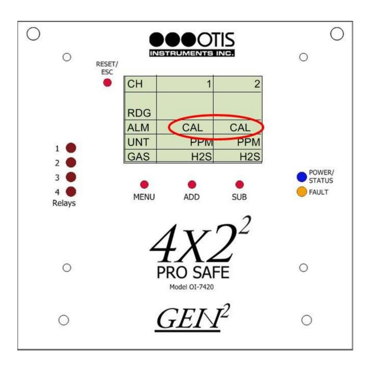
4. To return to Normal Operating Mode, press *RESET/ESC*.
