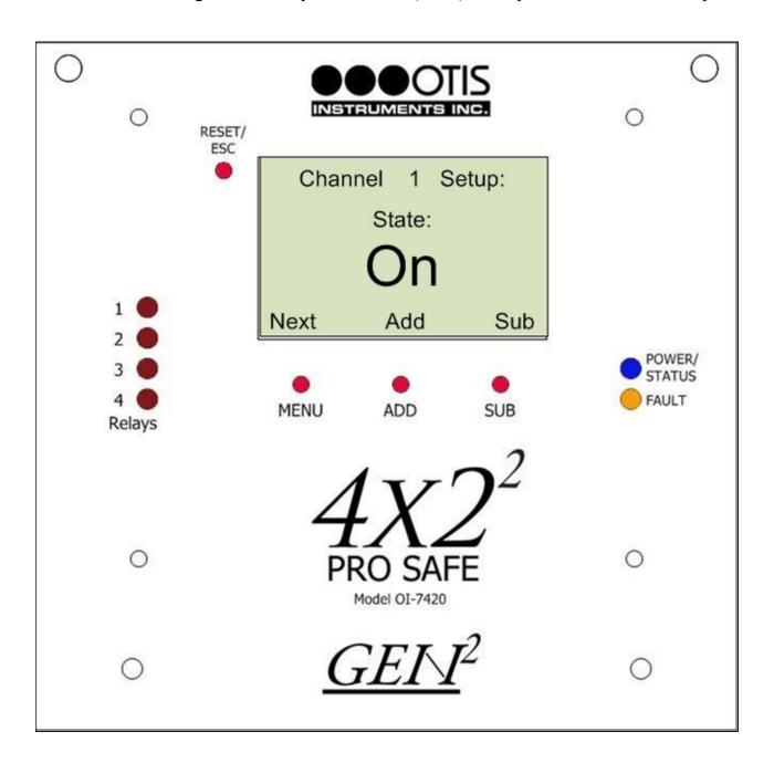
NOTE: All channels must be setup as On/Off before the information screen is available. If the channel is set to "On", additional settings will be available to set. If the channel is set to "Off", there will be no additional settings available for that channel, and pressing MENU will allow the user to move to the next channel to be set to On/Off. Once both channels are set, press MENU once more to view System Information (see page 37).
