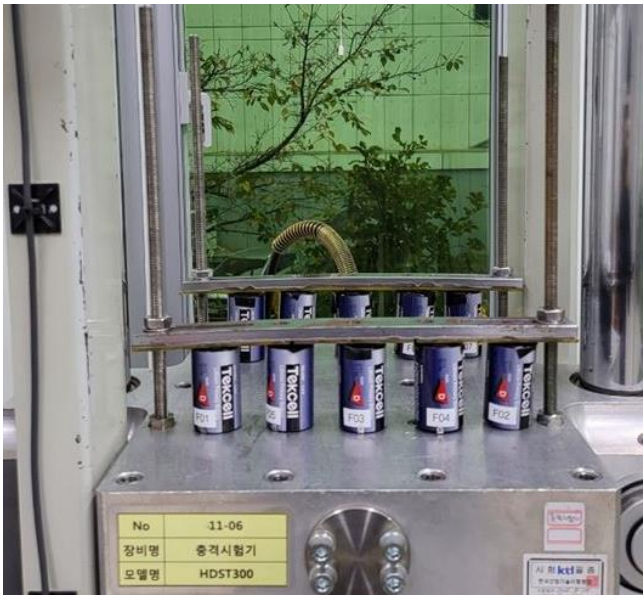
Photo.07 – Photographs of specimen before & after Shock test (Undischarged cells)
