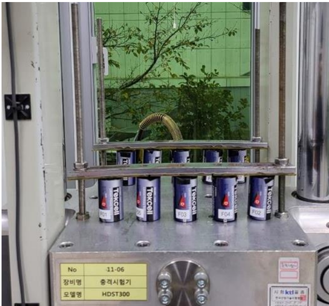
Photo.08 – Photographs of specimen before & after Shock test (Fully discharged cells)
